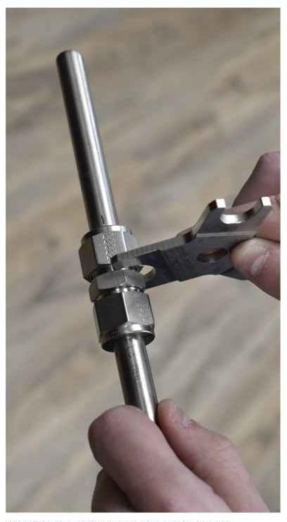
When fitting is properly tightened, gap gage should not fit between nut and shoulder of body.
