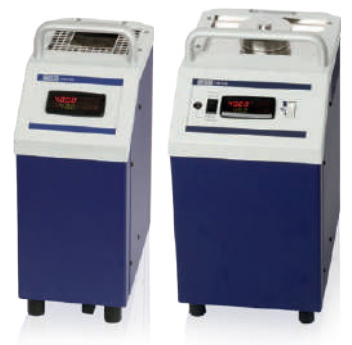
Dry-well calibrators for various temperature ranges
