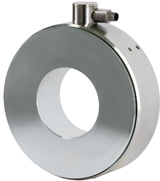
▲ Hydraulic ring force transducer with integrated pressure sensor and electrical output of 4 ... 20 mA.
